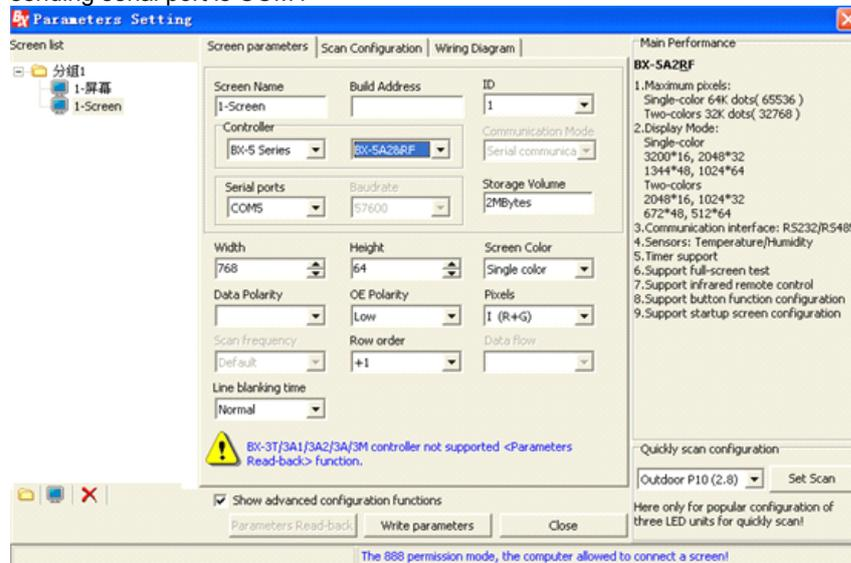
3. Installing LedshowTW 2012 graphic editor software (which has been installed, click directly), click set → set screen parameters → password: 168 → on the pop-up dialogue box (controlling assemblies)
